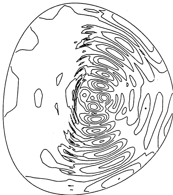
FIGURE 3. Distribution of the electric field produced in a cross section of a tokamak plasma irradiated by waves in the ion-cyclotron frequency range.
